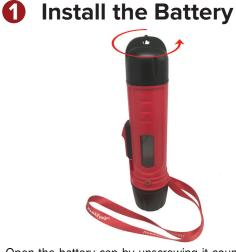
Open the battery cap by unscrewing it counter-clockwise. Plug a fully charged 9-Volt battery into the battery snap connector. Insert the snap connector and battery into the depth finder housing. Install the cap by turning clockwise until snug (do not over-tighten). Read the User's Guide
